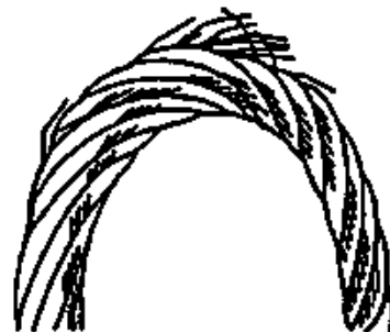
Band rope sharply to expose breakage
