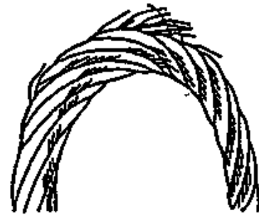
Bend rope sharply to expose breakage
